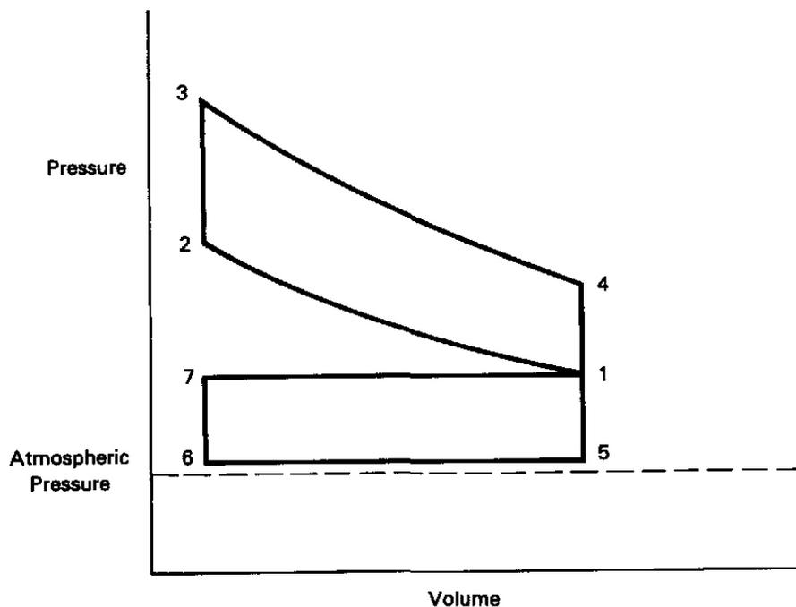
**FIGURE 6.11** Supercharged Otto cycle.
