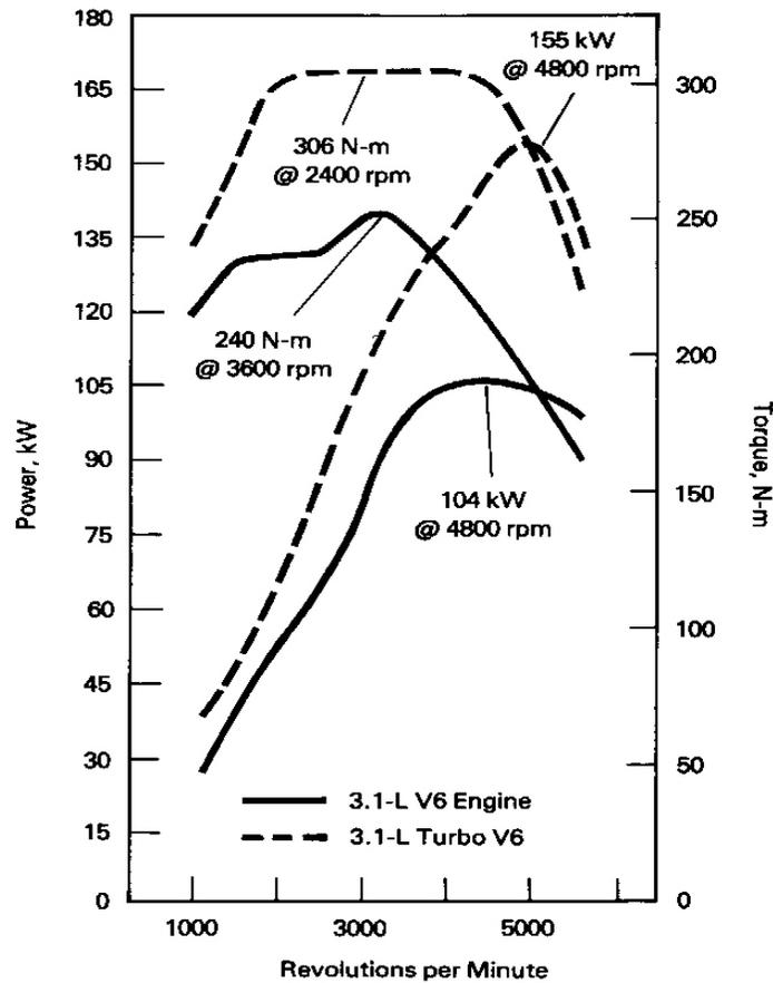
**FIGURE 6.8** Comparison of normally aspirated and turbocharged 3.1-liter engines. (Reprinted with permission from *Automotive Engineering* magazine, October 1988. Society of Automotive Engineers.)
