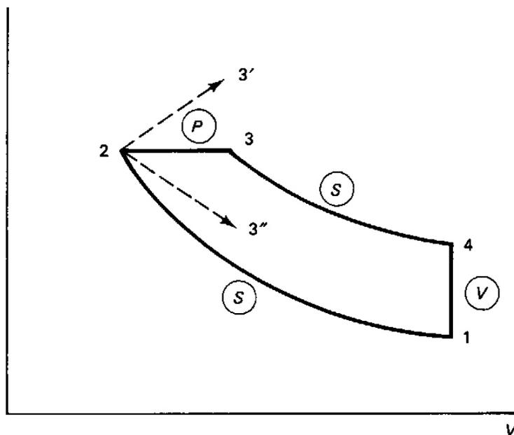
**FIGURE 6.9** The diesel cycle.
