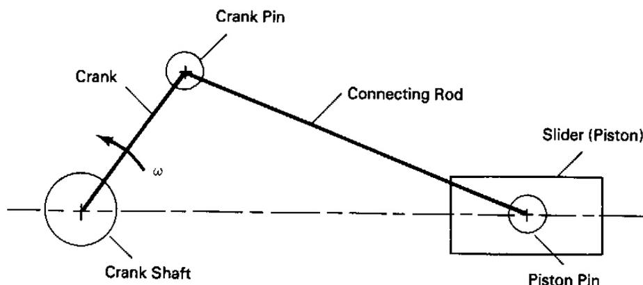
**FIGURE 6.1** Crank-slider mechanism.
